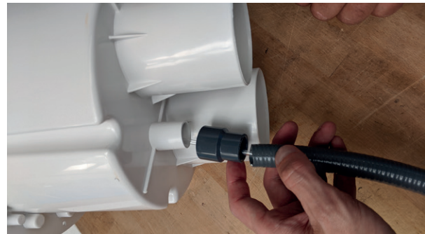
Outlet of the switching hose from the swim jet body via the reducer to the protective hose
