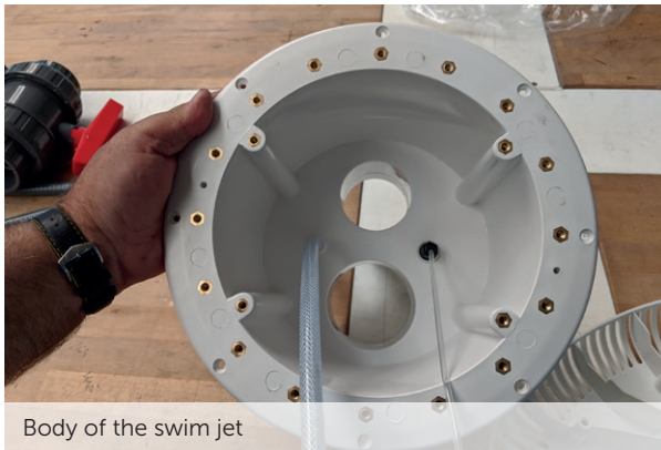
Outlet of the switching hose from the swim jet body via the reducer to the protective hose
