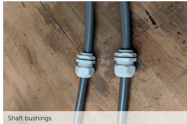
Outlet of the switching hose from the swim jet body via the reducer to the protective hose
