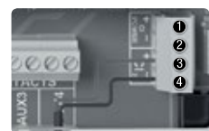
Free Chlorine probe ③ red ④ black
