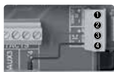
Free Chlorine probe ③ red ④ black
